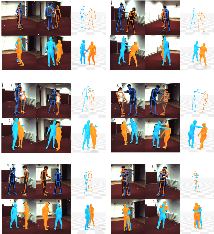
Fig. 7: Additional Qualitative Results. We show additional qualitative results of our method on the CHI3D dataset [6]. The left and middle columns show the 2D projections of the estimated 3D skeletons and SMPL body meshes on two views. The right column demonstrates skeletons and SMPL bodies in 3D scenes.
